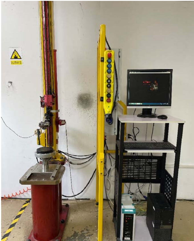
Impact attenuation test apparatus and data acquisition equipment
